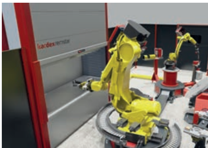
SHELF BACKSIDE Handling robot loads and unloads the trays
